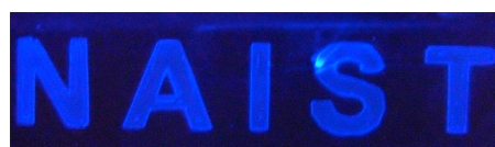
Fig. 7. Photopatterned film of poly(methyl methacrylate) containing 90a . The irradiated areas turn fluorescent because of the photoinduced conversion of non-fluorescent 90a to highly fluorescent 91a .
