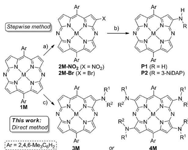
**Scheme 1.** Synthesis of amino-DAPs. a) Nitration (to **2M-NO<sub>2</sub>**) or bromination (to **2M-Br**); b) reduction (from **2M-NO<sub>2</sub>** to **P1**) or N–C cross-coupling (from **2M-Br** to **P2**); 3-NiDAP = 10,20-dimesityl-5,15-diaza(nickel)porphyrin-3-yl. c) Base-promoted direct substitution with amines (this study).
